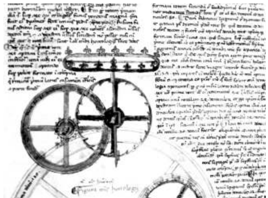
Fig 2. Giovanni Dondi's drawing 5 of the mechanism of his astronomical clock that he completed in 1364 that shows the balance-wheel in the form of a King's Crown.
